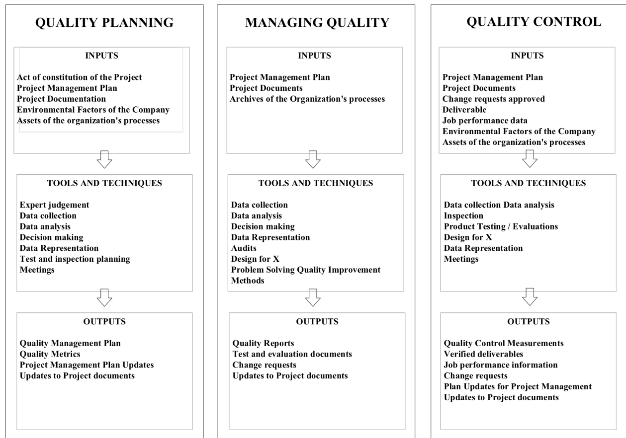
Figure 1. Processes for the quality management of a project according to PMBOK (Project Management Institute, 2017)
