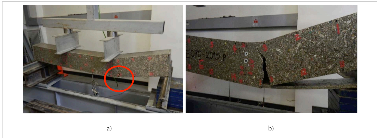
Figure 6. a) Hollow RTPBB-structural element typical crack beginning in a lower screw, b) Final failure stage for the beam, where crack advances into compression side of the lateral board
