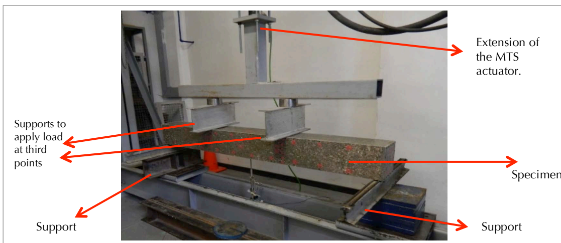
Figure 3. Specimen under bending tests using a central two-point load setup
