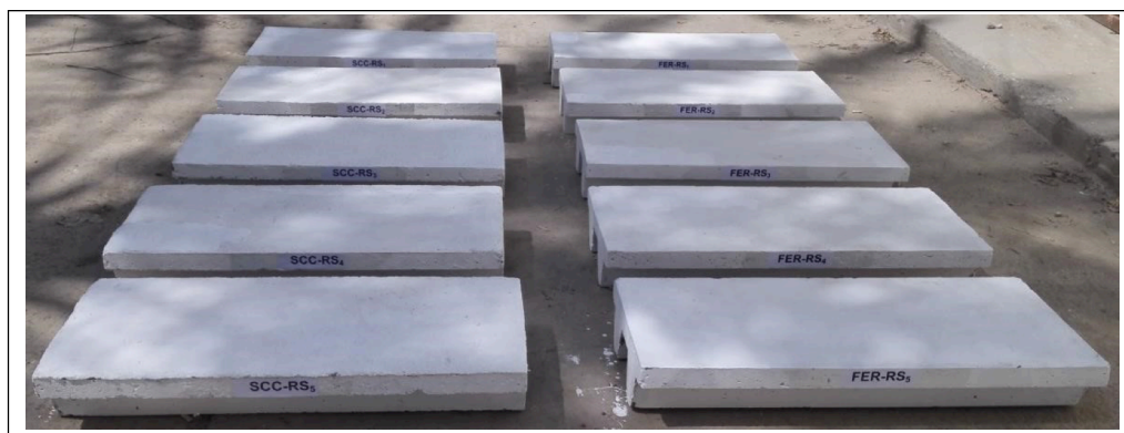
Figure 4. Ribbed panels after casting
